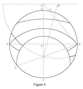
Having thus dispatched with the chore of drawing date curves, we now turn to the hour curves. Set off arc *EG* from *E* towards *C* equal to the latitude, and draw line *BG* (Figure 4). This is equivalent to setting  $\angle CBG = (90^{\circ} - \varphi)/2$ . Let *I* be the intersection of *BG* with *DE*. Point *I* will serve as the north pole of this projection; all hour curves will pass through it.
